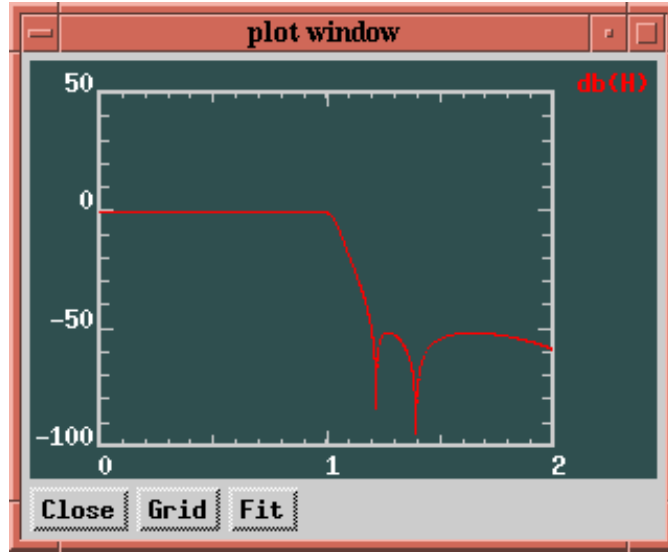
Figure 10: The transfer function of Figure 9 through xplot .
